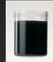
Black iron oxide sludge is deposited in a container.
