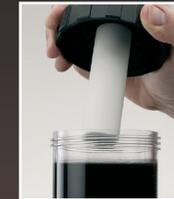
The *MagnaClean* filter is placed into the container...
