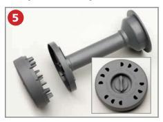
Unlock the bayonet screw on the base of the sheath and remove the debris collector. Rinse until all the non magnetic debris has been removed. Replace and lock the bayonet screw onto the sheath and place the sheath into the canister. Insert the magnet lid assembly and tighten until sealed.
