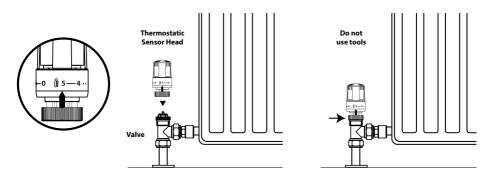
Figure 3.0 Sensor head Installation
