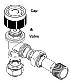
2. Screw the tail piece onto the radiator, slide on the nuts and olives and then fit the valve.
