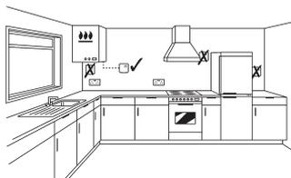
**GB** For best performance, install in an open space. Leave at least 30cm distance from any metal objects including wall boxes and boiler housing. **Do not mount on metal wall boxes.**
