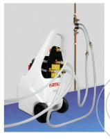
A pair of 0.5 metre long adapter hoses, enabling the pump to be connected across the 1½" unions, are supplied as standard. When used, these are screwed directly onto the ¾" female brass hose adaptors of the flow and return hoses, giving a total hose length of 5.5 metres.
