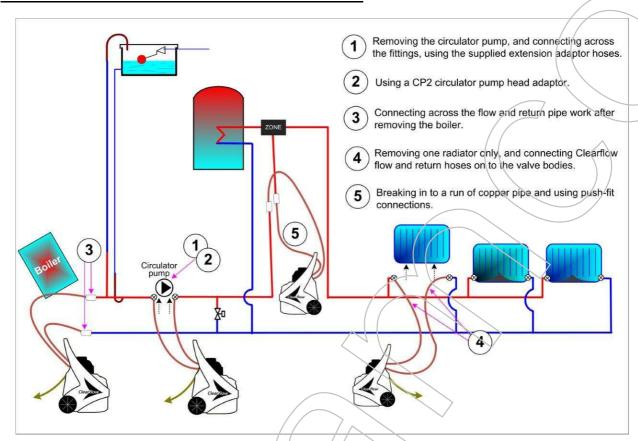
The connection point for the flushing pump may vary depending on the system to be cleaned, and the availability of suitable connection points.
